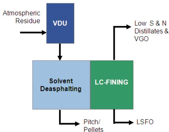
**Figure 5: SDA Upstream of an LC-FINING Unit**
