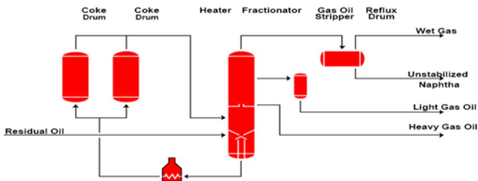
**Figure 2: Schematic of a Delayed Coking Unit**
