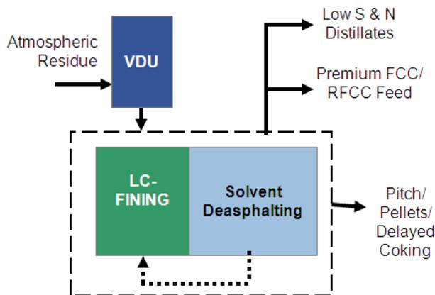
Figure 6: SDA Downstream of an LC-FINING Unit
