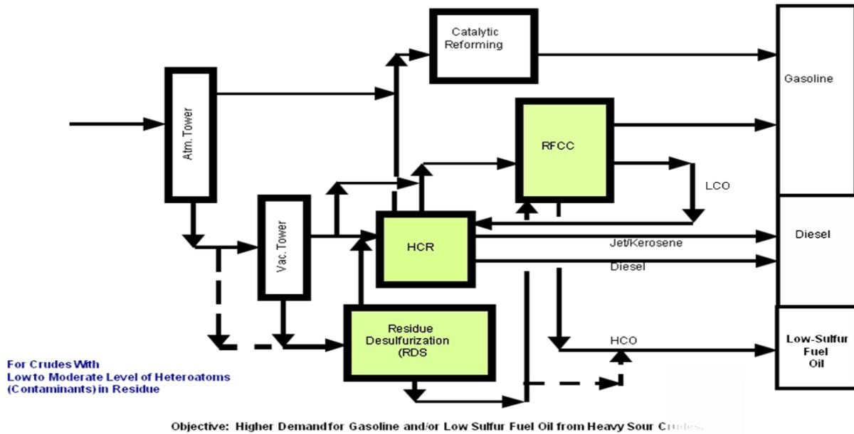
**Figure 11: Refinery Scheme With RDS as Residue Upgrader**
