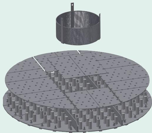
Figure 1: Inlet distribution basket and top nozzle tray assembly
