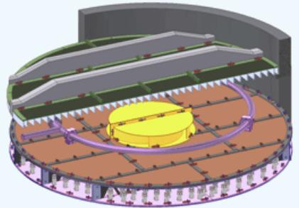
ISOMIX<sup>®</sup>-e utilizes an optimum truss system structure to support the internals components while the beams holding up the catalyst support panels are oriented upward to increase the catalyst volume.
