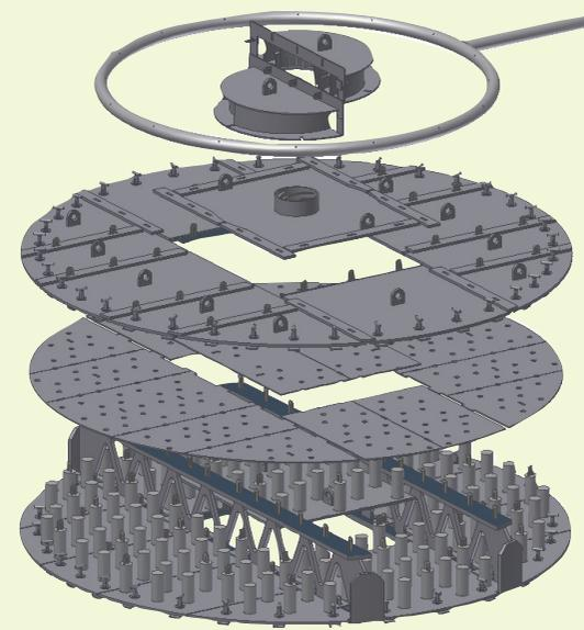
Figure 3: Interbed reactor internals
