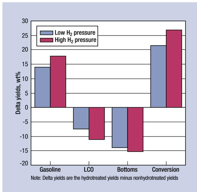
**FIG. 1** Benefits of FCC pretreating—hydrotreated feed vs. nonhydrotreated feed.
