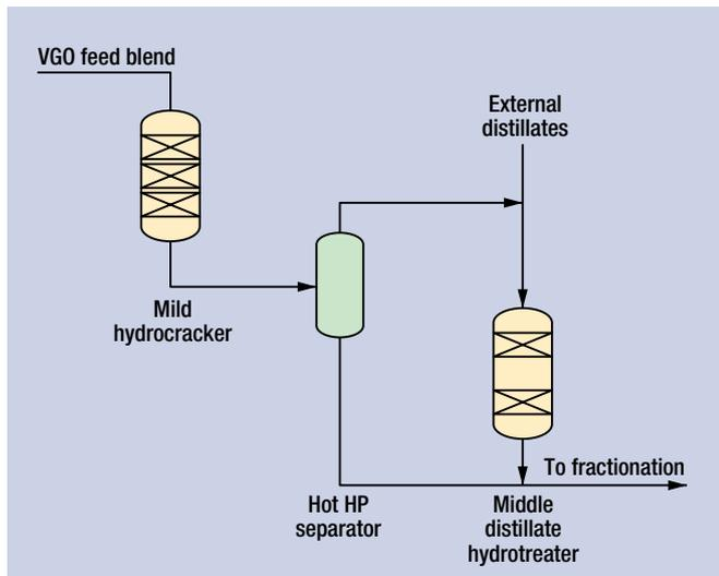
**FIG. 8** The two-step mild hydrocracking process and middle-distillate hydrotreating process.
