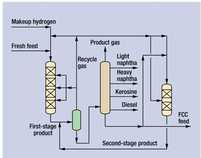
**FIG. 9** Optimized partial-conversion hydrocracking process for heavy feeds—HCGO/HVGO/FCC LCO blends.
