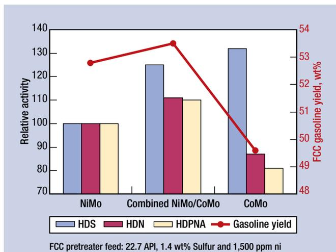
**FIG. 2** Activity and gasoline yield using the combined NiMo/CoMo catalyst system to hydrotreat coker gasoil for FCC pretreatment.
