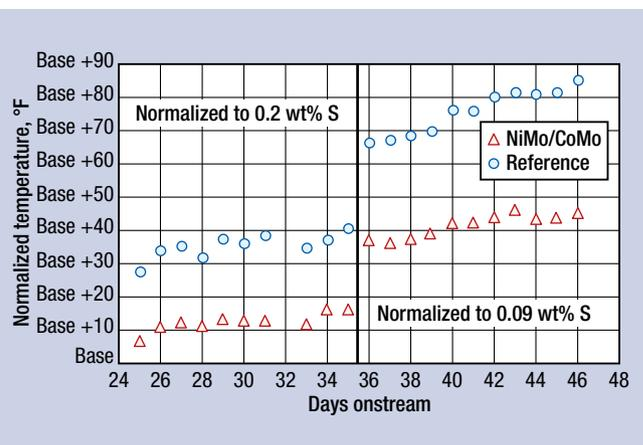
**FIG. 5** Hydrosulfurization activity for of the NiMo/CoMo catalyst system treating a DAO containing feed.
