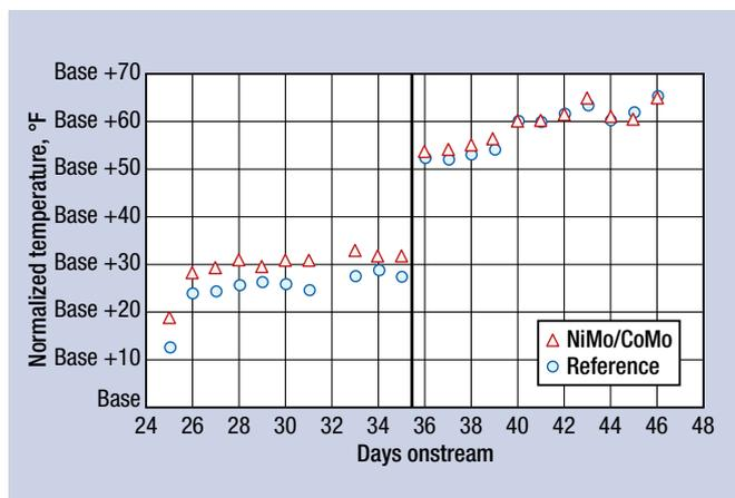
**FIG. 6** Hydrodenitrification activity of the NiMo/CoMo catalyst system treating a DAO containing feed.
