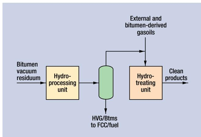
**FIG. 7** Integrated hydroprocessing/HDT scheme to upgrade Alberta bitumen.
