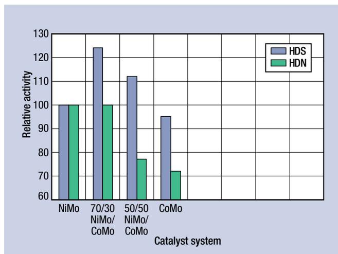
**FIG. 3** Activity of using combined NiMo/CoMo catalyst systems to hydrotreat HCGO/VGO blends at high pressure conditions.
