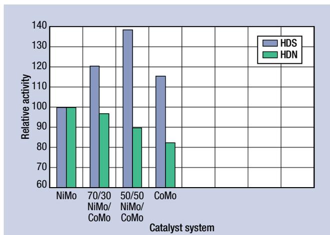
**FIG. 4** Activity of using combined NiMo/CoMo catalyst system to hydrotreat HCGO/VGO blends at low pressure system conditions.
